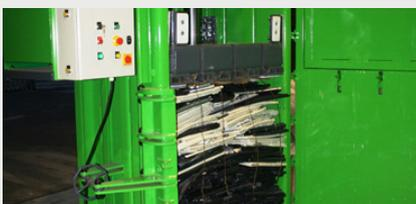
Extra-long stroke ram and extra retention fingers for optimal compaction and heavy-duty wire tie
