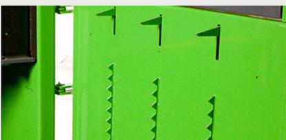
Unique configuration of floating and fixed retention fingers helps optimise baling
