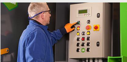
Automatic cycle with "Bale Full" indicator light and anti-jam programme for safe operation
